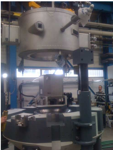
Assembly of the magnet inside the yoke at the Customer's site
