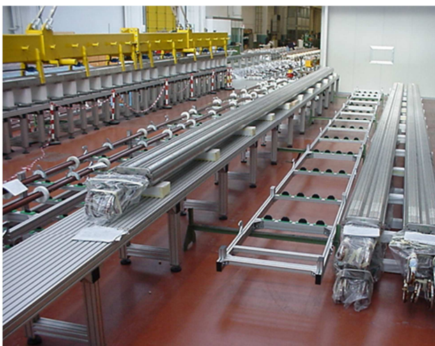
Collared coils completed
