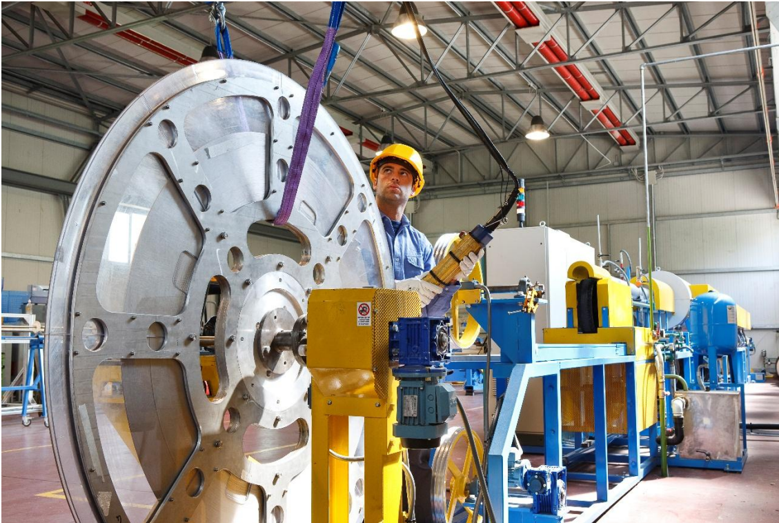
A technician working on MgB 2 superconducting wire at the ASG facilities.
