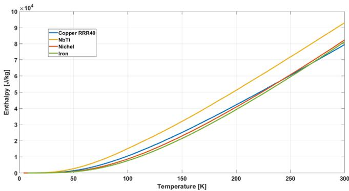
Figure 1 Example of enthalpy for typical materials used in superconductor manufacturing
