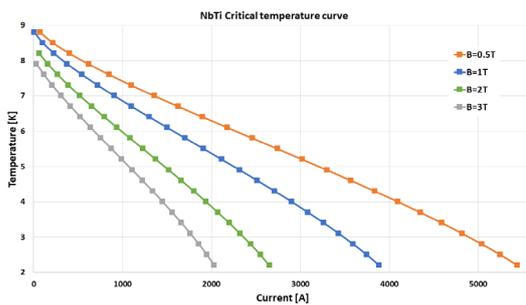
Figure 15 Critical temperature curve of NbTi standard Ø1.8
