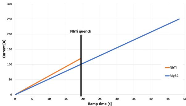
Figure 9 Recorder current during maximum speed ramp
