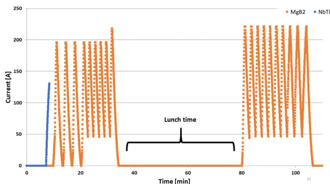
Figure 18 Recorded current during multiple ramp up
