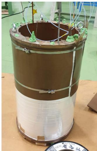
Figure 7 Photo of the coil before the impregnation process
