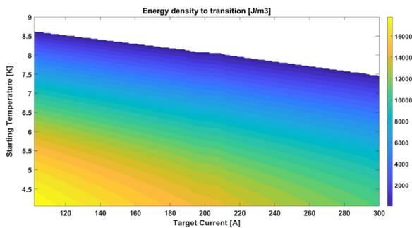
Figure 13 Energy density to transition for NbTi winding as function of starting temperature and target current (adiabatic conditions)
