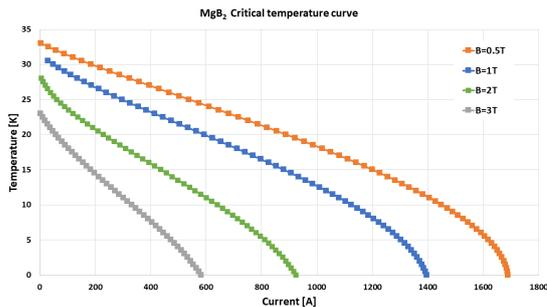
Figure 14 Critical temperature curve of MgB<sub>2</sub> MRO plus wire
