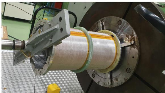
*Figure 6* Photo of the former placed on the winding machine with counter mass and G10 shoulders
