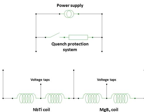
Figure 5 Electrical scheme of the experimental set up
