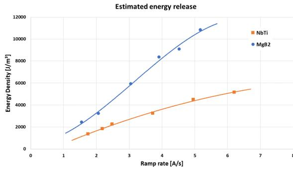
Figure 11 Energy release at different ramp rate
