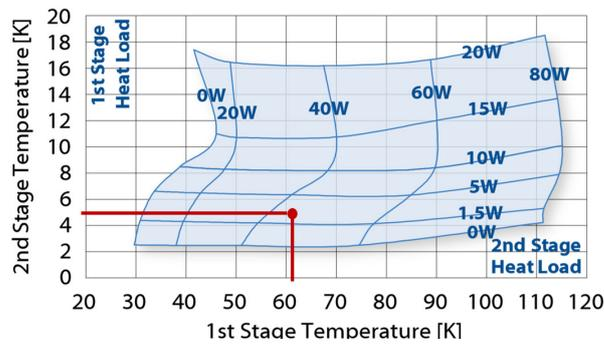
Figure 4 Capacity map of Sumitomo RDK 415D and operating conditions of the facility (in red)
