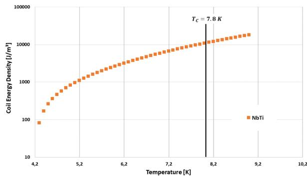
Figure 16 NbTi coil energy density as function of temperature
