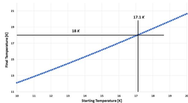
Figure 17 Relation between starting and final temperature of the MgB<sub>2</sub> winding during ramp up
