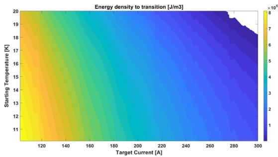
Figure 12 Energy density to transition for MgB<sub>2</sub> winding as function of starting temperature and target current (adiabatic conditions)
