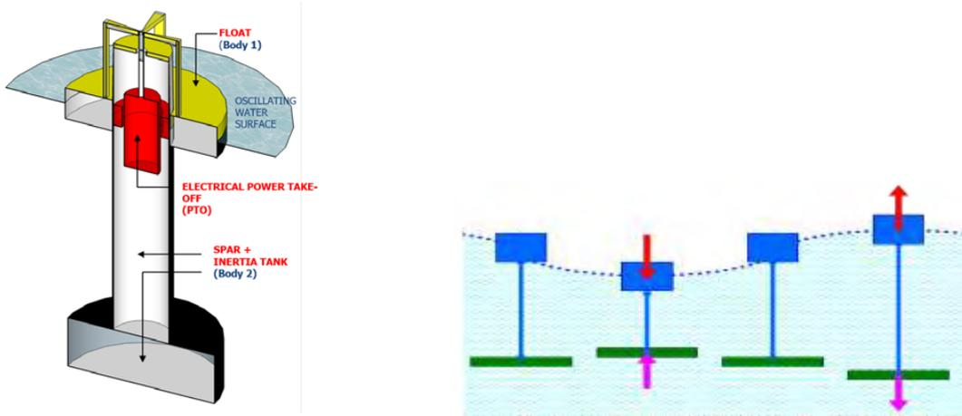
Figure 4 Configuration of a Heaving Point Absorber.
