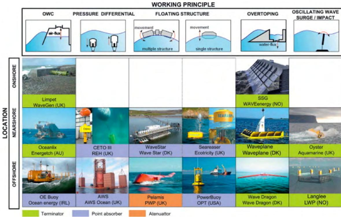
Figure 3 Classification of WEC typologies based on location and working principle.
