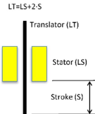
Figure 5 Direct-Drive machine scheme.
