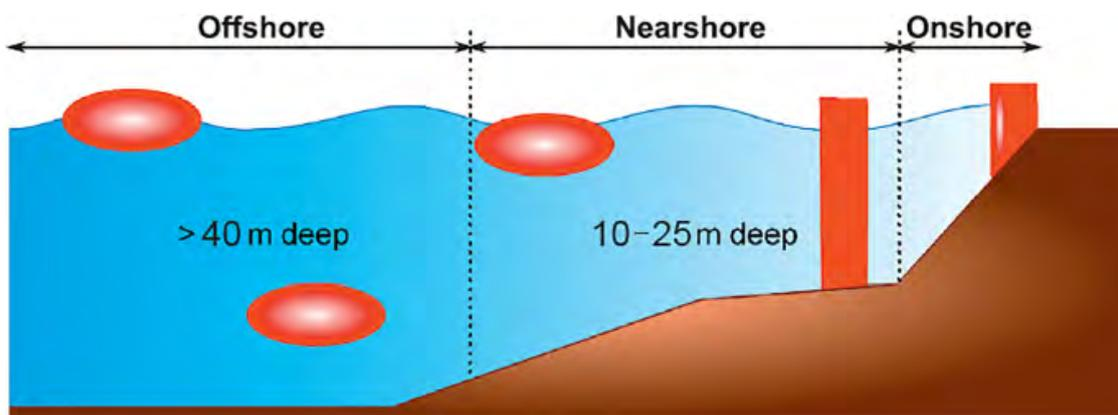
Figure 2 Classification of the WEC typologies based on location.
