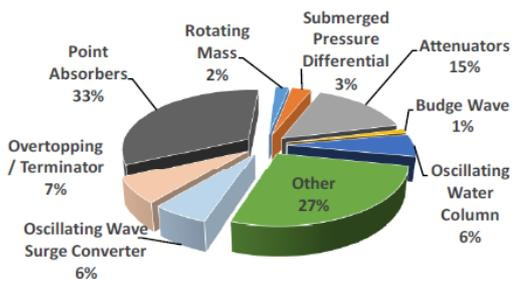
Figure 1 Different WEC typologies and their distribution rate.
