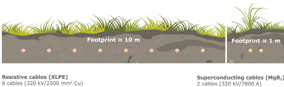
Fig. 8. Comparison of the environmental footprint of resistive XLPE cables and MgB<sub>2</sub> superconducting cables for a 6.4 GW DC power link.
