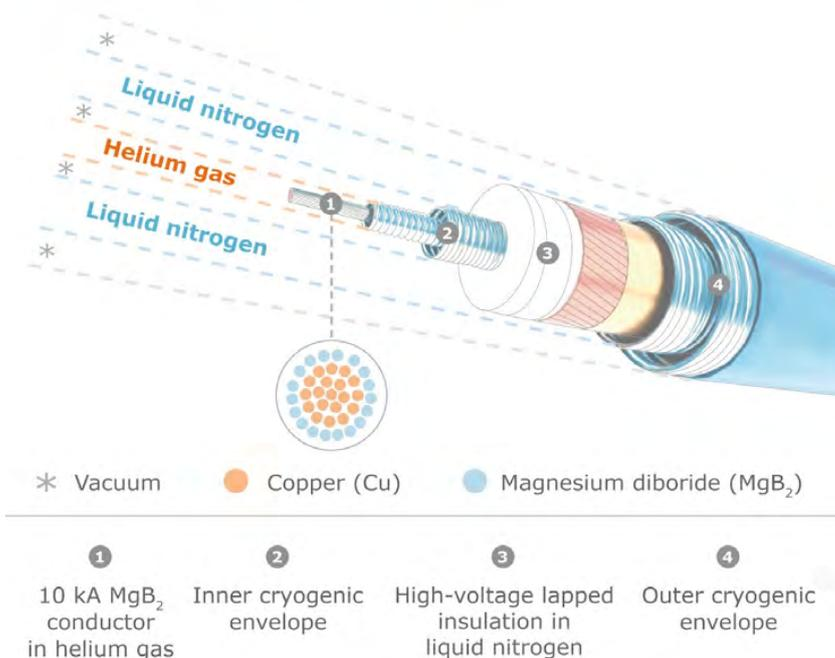
Fig. 1. Sketch of the 3.2 GW MgB<sub>2</sub> cable system showing the key components. The electrical terminations are not represented here.
