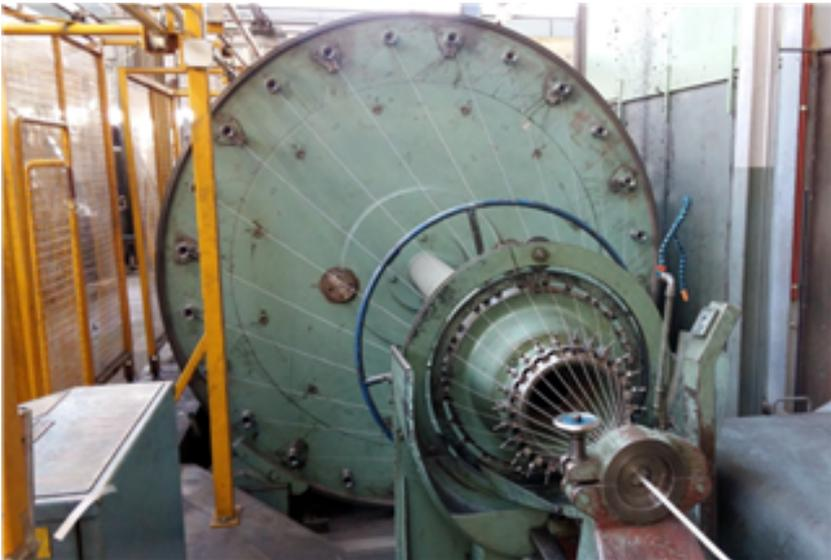
Fig. 3. Planetary cabling machine from Nexans used to manufacture the cable conductor for Best Paths (courtesy of Nexans).
