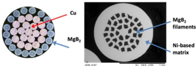
Fig. 2. Picture of the 10 kA cable conductor consisting of 18 MgB<sub>2</sub> wires wound around a copper core (left) and one MgB<sub>2</sub> wire composed of 36 superconducting filaments embedded in a matrix of nickel and monel (right).
