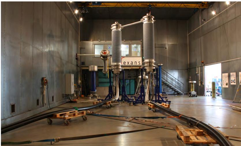
Fig. 6. Testing loop shown together with the 800 kV DC generator on the Nexans testing platform (courtesy of Nexans).
