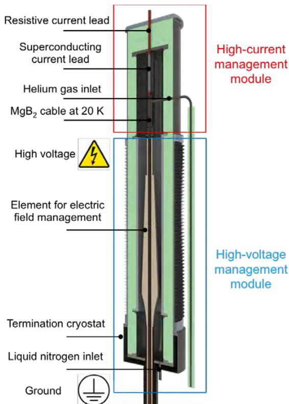
Fig. 5. Sketch of the HVDC termination developed for Best Paths, highlighting its modular design.
