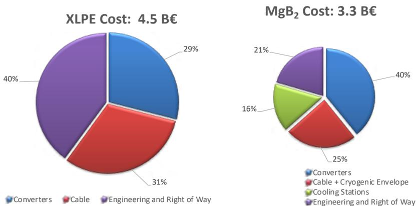
Fig. 7. Capital costs of resistive XLPE cables and MgB<sub>2</sub> superconducting cables for a 6.4 GW DC power link with a length of 500 km.
