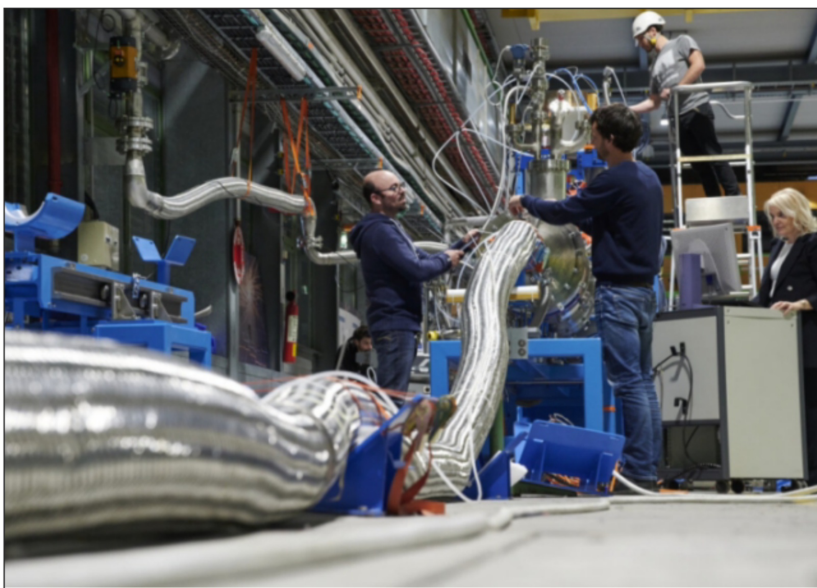
WIRES FOR HIGH CURRENT LINKS Advanced superconducting wire for high current links
