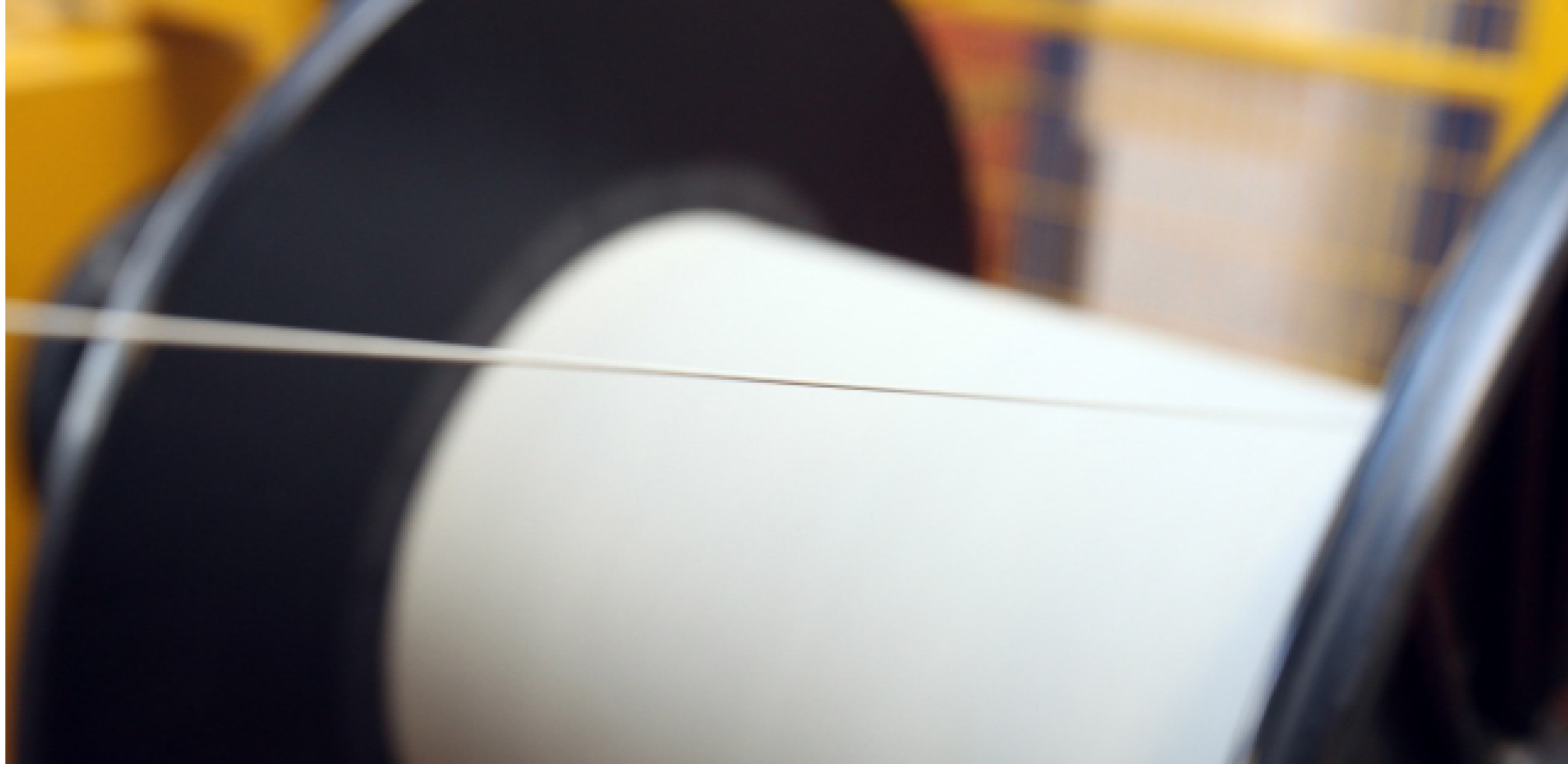
MRO PLUS WIRE FOR CRYO-FREE MAGNETS Improved multifilamentary superconducting tape for higher field magnets
