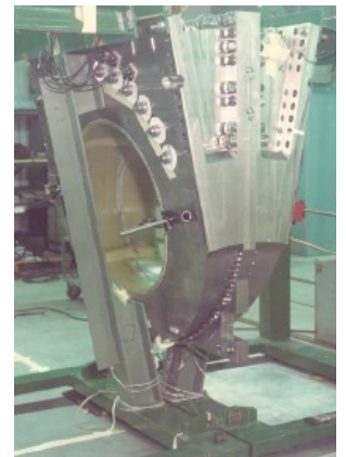
Shrink fitting assembly of one toroidal coil module
