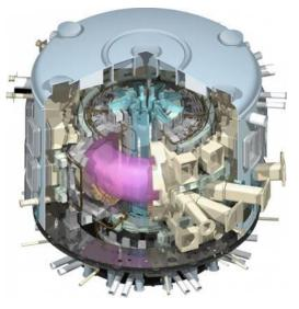
The fusion process involves two hydrogen isotopes, deuterium and tritium, heated to temperatures in excess of 150 million °C, forming a hot plasma. Strong magnetic fields are used to keep the plasma away from the walls; these are produced by superconducting coils surrounding the vessel, and by an electrical current driven through the plasma.
